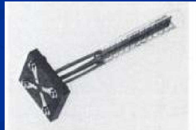
Figure 9 The temperature-sensing end of a resistance thermometer
