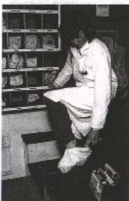
▲ This nuclear laboratory worker is about to use a GM tube and ratemeter to check for any traces of radioactive dust on her clothing.
