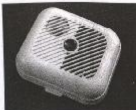
Smoke detectors contain a small amount of americium-241, an alpha emitter. When smoke (or other invisible products of combustion) enters the detector it reduces the number of alpha particles reaching an electronic detector. This triggers an alarm.
