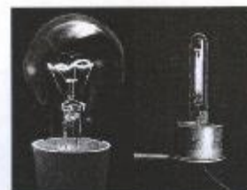
A filament lamp (left), emits the characteristic continuous spectrum of a hot solid and a significant amount of its energy is in the infrared part of the spectrum. In a strip light (right), mercury vapour is excited by passing a current through it. It then emits visible and ultraviolet radiation. Sometimes the inside of the tube is coated with fluorescent material that converts the ultraviolet to visible radiation, providing an efficient source of white light.
