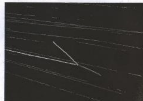
Tracks of alpha particles in a cloud chamber. The colours are false and have been added to the picture. The green and yellow lines are the alpha tracks. The red line is the track of a nitrogen nucleus that has been hit by an alpha particle.
